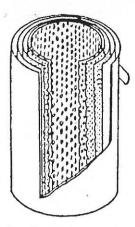
Dimensions in cm: External diameter: 43 Diameters of screens: 18, 23, 28, 33
